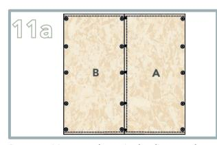
Screw positions are shown in the diagram above. The larger screw heads are 125mm and the smaller ones are 35mm. The final floor result should now be fully secured and flush around all faces of the bearers beneath. Use spirit level to ensure the floor is level before continuing with the build.
