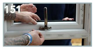
Apply the window handle with the screws provided. Remove the hole caps and drill the screws into the space provided. Then cover the holes back up with the caps.
